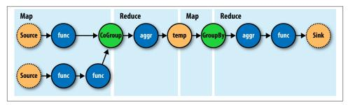
Figure 24-8. How a Flow translates to chained MapReduce jobs
