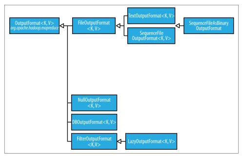
Figure 8-4. OutputFormat class hierarchy
