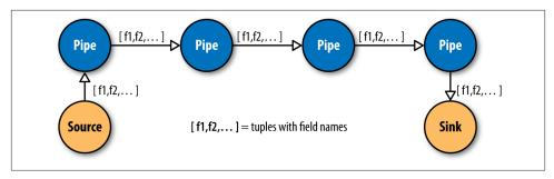
Figure 24-2. Pipes linked by fields and tuples
