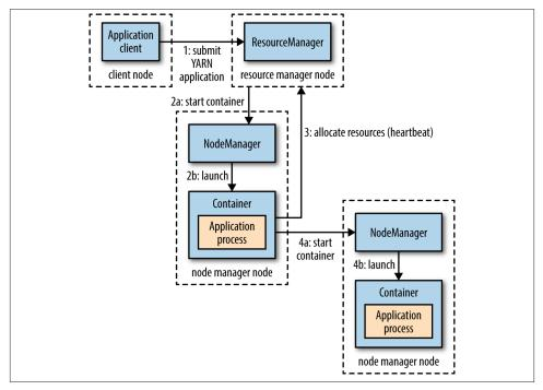
Figure 4-2. How YARN runs an application
