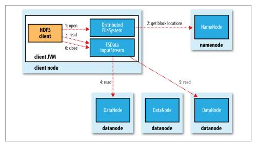
Figure 3-2. A client reading data from HDFS
