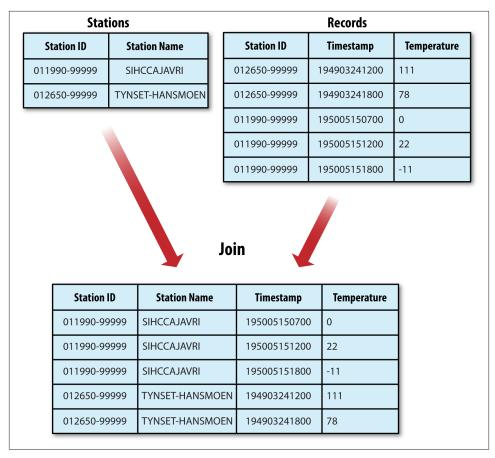
Figure 9-2. Inner join of two datasets
